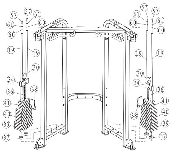
STEP 3 Slide the Guide Rods (19) into the holes located on the Left and Right Frames (1 & 2). Now apply the Lithium Grease included with your bolt pack onto the Guide Rods (19).
